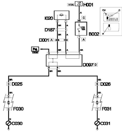
Component codeDescriptionReference to the assemblyB002JUNCTION UNIT UNDER DASHBOARD-C030LEFT REAR EARTH-C031RIGHT REAR EARTH-
