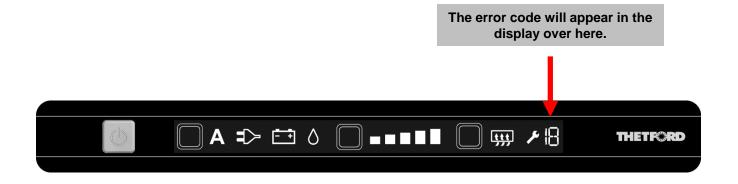
III Note : When supply voltage 12 VDC (low current voltage) is not available, no error code will be given. When 12VDC is available the green power LED will be on III
