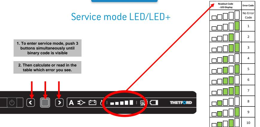
III Note : When supply voltage 12 VDC (low current voltage) is not available, no error code will be given. When 12 VDC is available the green power LED will be on. If battery pack is empty you can see a red light !!!
